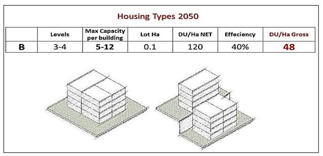
Figure 8-3 Housing Type B
